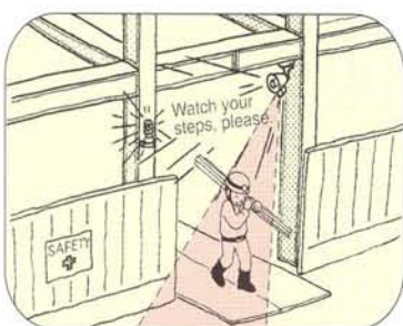
● Alarm/warning speaker at construction site
